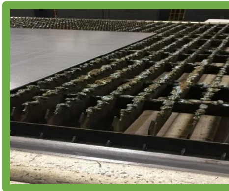
Enough amount of slag for cleaning
